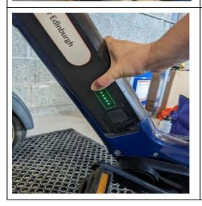
3) To check if the battery is fully charged: Hold down the power button on the battery for around 2 seconds to switch it on. Press the power button once again to see the charge level. Five green LED lights mean the battery is fully charged.
