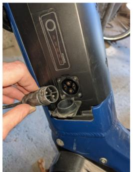
2) Simply plug one of the cables attached to the wall into the port on your bike's battery.
