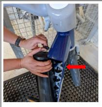
**3A)** Hold the key in the twisted clockwise position. Grasp the top of the battery and pull towards yourself. The battery should slide out to the left of the bike.
