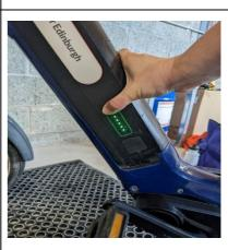
**8)** Hold down the power button on the battery for around 2 seconds to switch it on. Press the power button once again to see the charge level. Five green LED lights mean the battery is fully charged.
