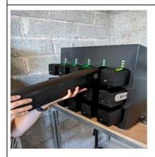
**6)** If there is a charged battery available, take it and put it in your bike. Put the old battery into the space in the charger to recharge. It might be that no fully charged batteries are available – if so, remove your bike's battery and put it on to charge, then replace it again later.
