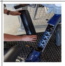
**4)** Remove the battery and place it on the mat.
