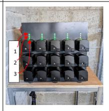
**5)** The lights on the charging unit indicate whether a battery is fully charged (green) or charging (red). The lights correspond to each battery in that column. Batteries take 4 hours to fully charge.
