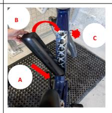
7) Insert the freshly charged battery into the bike. Place the bottom of the battery in first (A) and then slide the battery in from left to right (B). When the battery is fully inserted, you should hear a clicking noise (C).
