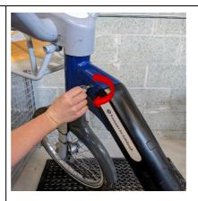
**2)** Place your bike on the mat at the side of the charging area. Locate the key from inside the charging area. Insert the key and twist clockwise.
